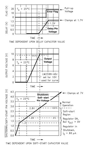
Figure 29. Soft-start, Delay, Error, Output
