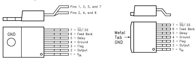
Figure 1. Bent and Staggered Leads, Through
