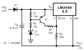
Figure 47. Undervoltage Lockout Without Hysteresis for an Inverting Regulator
