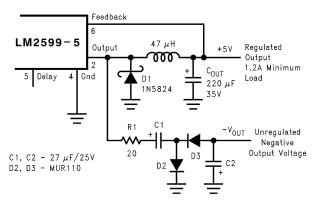
Figure 49. Charge Pump for Generating a Low Current, Negative Output Voltage
