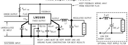
Component Values shown are for  $V_{IN} = 15V$ ,
