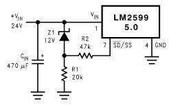
Figure 46. Undervoltage Lockout for a Buck Regulator
