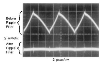
Figure 36. Post Ripple Filter Waveform
