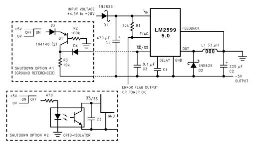
Figure 43. Inverting -5V Regulator With Shutdown and Soft-start
