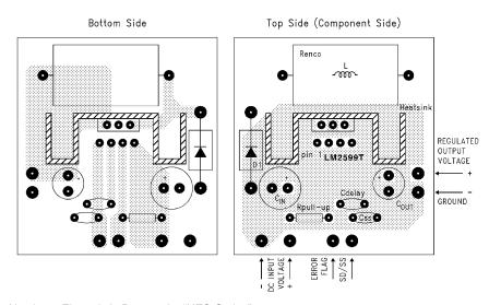
$C_{\text{IN}}:~-470~\mu\text{F},\,50\text{V},\,\text{Aluminum Electrolytic Panasonic, "HFQ Series"}$
