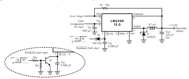
Figure 42. Typical Circuit Using Shutdown /Soft-start and Error Flag Features
