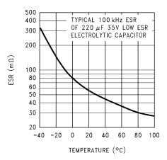
Figure 34. Capacitor ESR Change vs Temperature
