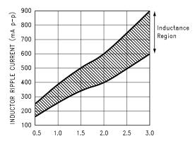
Figure 37. Peak-to-Peak Inductor Ripple Current vs Load Current
