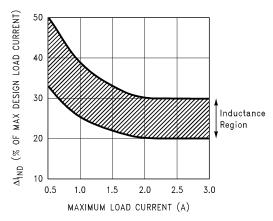
Figure 35. (ΔI<sub>IND</sub>) Peak-to-Peak Inductor Ripple Current (as a Percentage of the Load Current) vs Load Current
