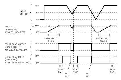
Figure 30. Timing Diagram for 5V Output
