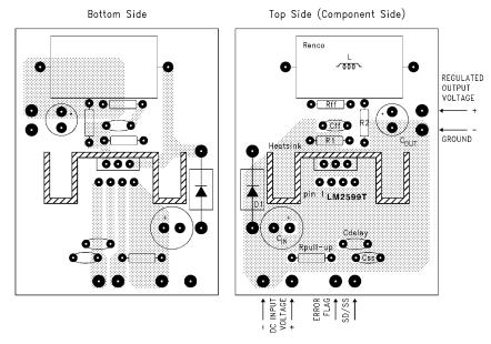
$C_{IN}$ : — 470  $\mu$ F, 50V, Aluminum Electrolytic Panasonic, "HFQ Series" C<sub>OUT</sub>: — 220 μF, 35V Aluminum Electrolytic Panasonic, "HFQ Series"
